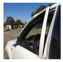
But even the best built vehicle and door design will need regular inspection and maintenance as to the how the door hangs and fits into the doorframe. The best way to do this is carefully watch the door as it closes and look for any vertical movement as the door itself moves into the doorframe.
